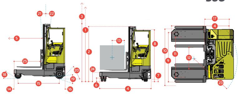
This compact truck features two rear wheel drive with rubber tyres and dynamic 360° steering rotation, contributing to faster procedures for manufacturing distribution and logistics operations.
